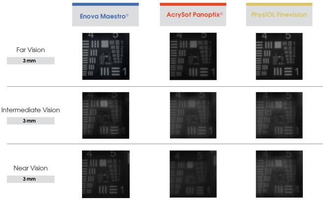
MeasurementEquipment: Lambda PMTF device (Belgium) with 3 and 4.5 mm / In-housemeasurement
